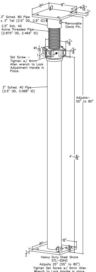
Tighten Set Screw w/ 6mm Allen Wrench to Lock Handle in place.
