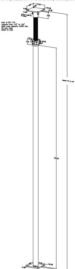
Use Turning Bar as lever for height adjustment (Item # MJ—TB12, MJ—TB24, MJ—TB36).
