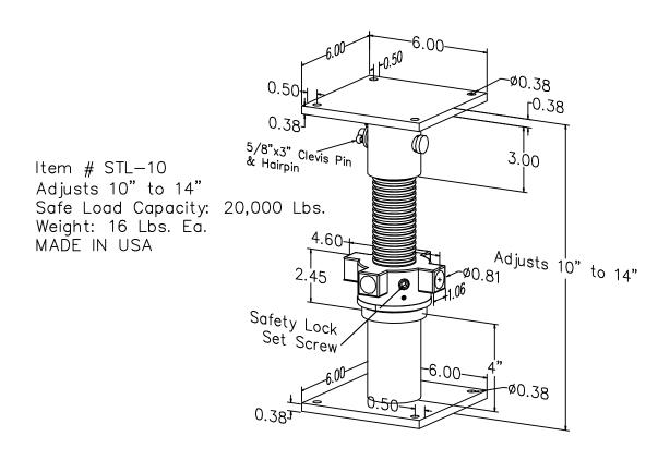
Use Turning Bar as lever for height adjustment (Item # MJ-TB12, MJ-TB24, MJ-TB36).
