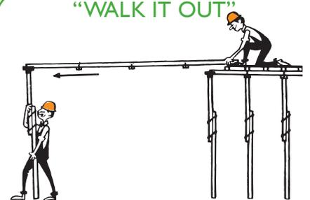
Man above pushes purlin end out, man below slips shore into purlin splicer, walk it out. Top man seats and nails it.
