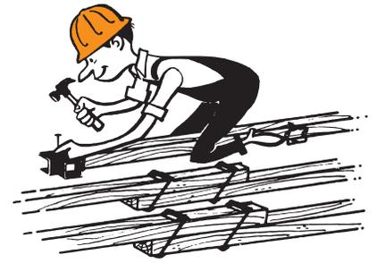
On ground, attach Ellis metal parts to lumber.
