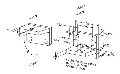
Plate Ear - 6" Tall Forging for HS-46 & HS-610
