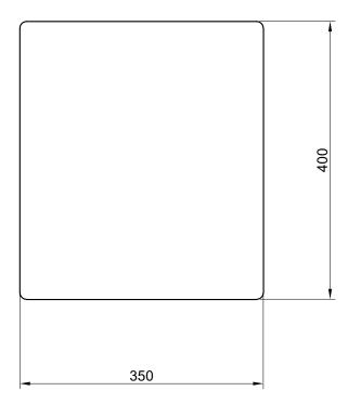
All measurements in millimetres
