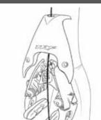
Install aero cover BEFORE installing cable in actuation wedge.
