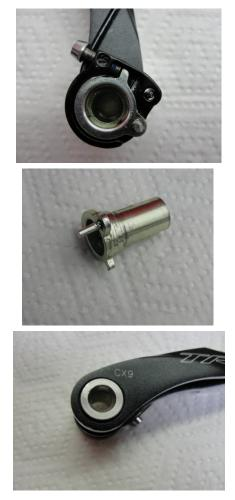
Apply an ample amount of grease to the bushing pivot barrel and reassemble the pivot bushing barrel and spring assembly.
