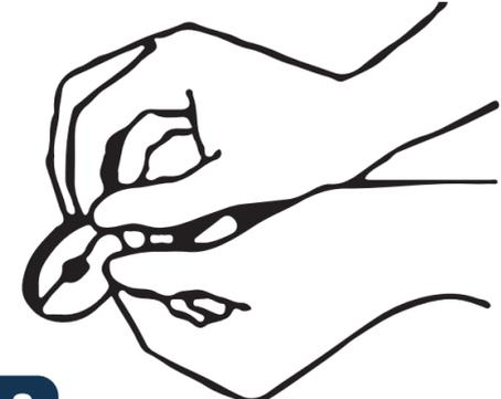
3 Place rubber sealing disks over each leg port, leaving screw hole exposed.
