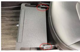
STEP 6 Push the safe completely under the seat
