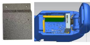
**STEP 5** Use the **punching cone** to poke four **holes** the inner wall of the armrest box through the reserved holes.
