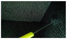
**STEPS 4** Use a Phillips screwdriver to tighten the self-tapping screws. Don't over-tightening the screws and over-tighten cause damage to the armrest box.
