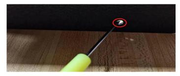
**STEPS 4** Use a Phillips screwdriver to tighten the self-tapping screws. Don't over-tightening the screws and over-tighten cause damage to the armrest box.
