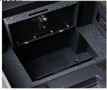
**STEPS 4** Use a wrench to tighten the bolts with the washers. Don't over-tightening the screws and over-tighten cause damage to the armrest box. Reinstall the plastic brackets.
