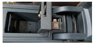
**STEPS 4** Ensure the reserved **holes** of the safe **line up** with the **holes** of the armrest box. **Hand the screws into the armrest box' holes via the reserved holes of the safe.** Use a wrench to tighten the factory bolts. **Don't over-tighten** the bolts, over-tightening will cause **damage** to the armrest box.
