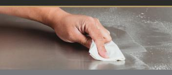
Use the correct tools, clean water and non-chloride cleaners to wipe off dirty stainless steel surfaces. Do not allow liquids, food particles, dirt, or foreign debris to stand on the stainless steel for prolonged periods of time. Do not use chlorine bleach. If used, rinse off with water immediately and wipe off surface with a soft clean towel.
