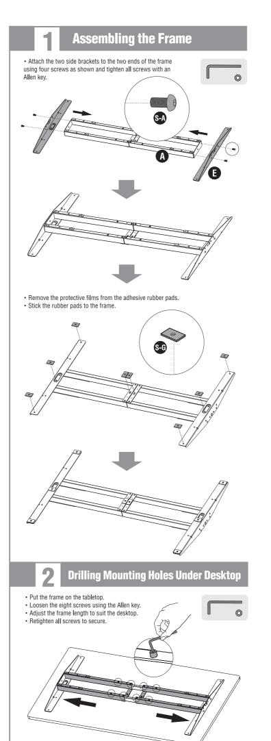
• Drill mounting holes under the desktop, then remove the desktop.
