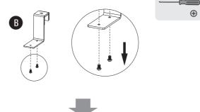
• Fix the hooks to the shelf with removed screws, tighten all the screws.
