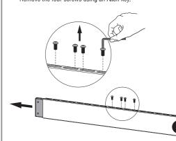
Adjust the crossbar to align with the lifting columns mounting holes and tighten the four screws to secure.
