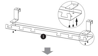
· Hang the cable management shelf onto the frame as shown below.
