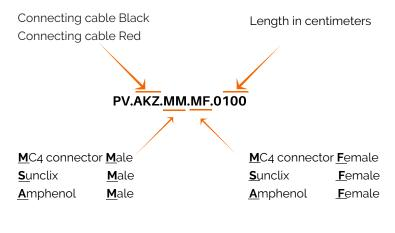
By using various connectors, it is possible to assemble the correct connection cables for each combination of PV box and converter.
