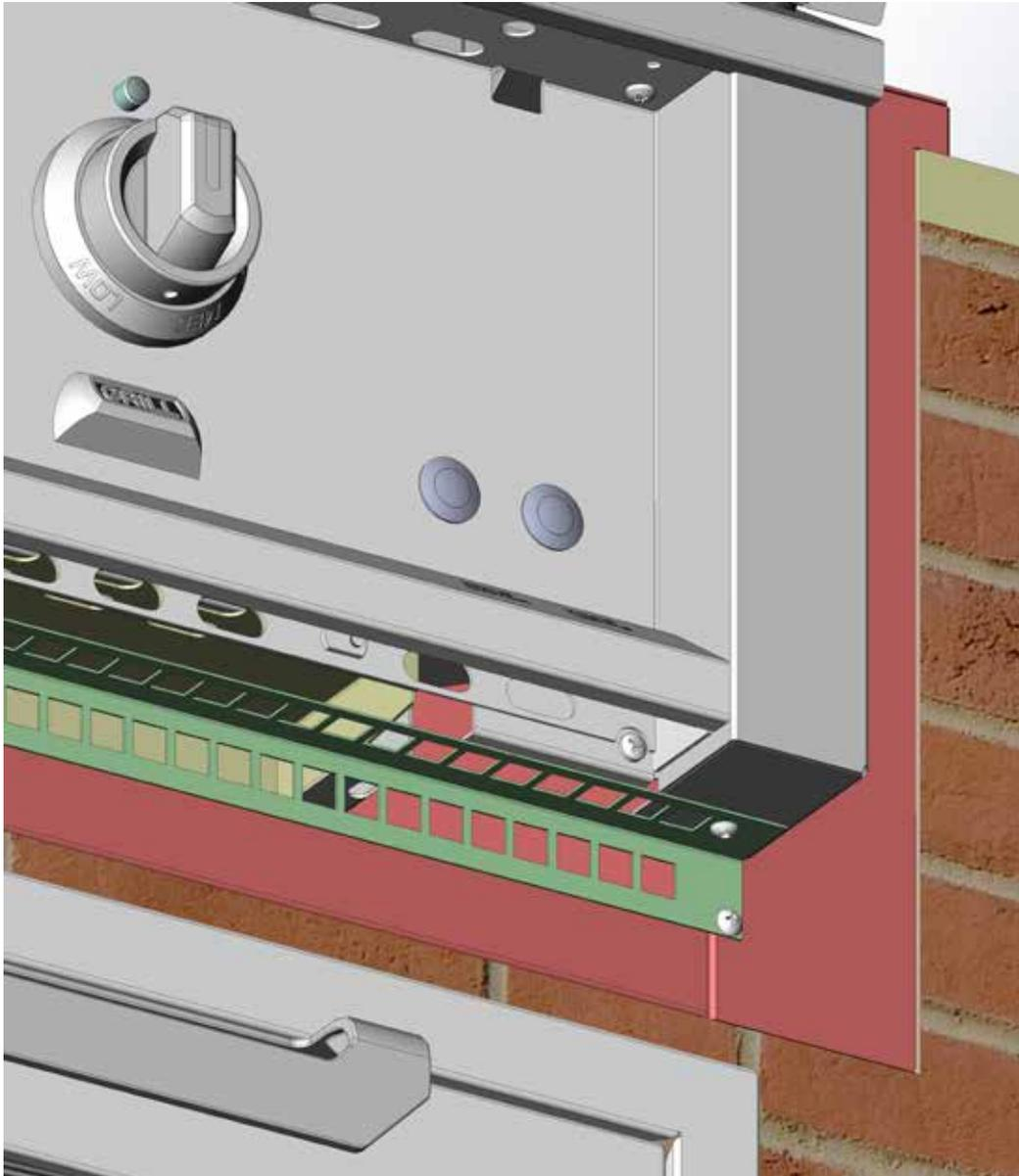
8. Proceed with the remainder of the grill installation as documented in the Use & Care Manual that came with your Hestan grill. Follow all instructions for regulator installation, gas connections, leak testing, burner adjustment, etc. before using your grill. After all these steps are completed, you can re-install the control panel and knobs.
