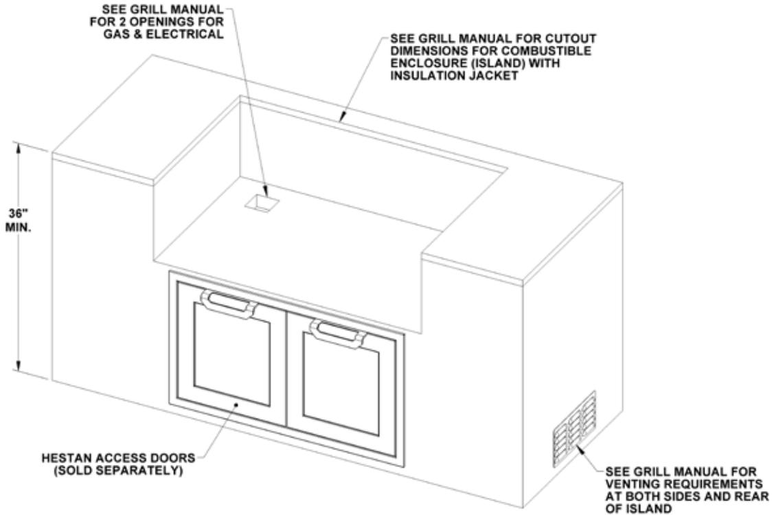
2. Slide in the Insulation Jacket as per the image below. The front face of the jacket should be flush to the face of your island.
