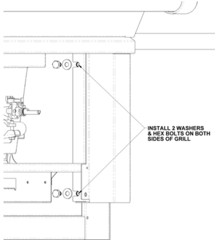
6. If needed, the rear of the grill can also be secured to the rear of the jacket. This step is optional.
