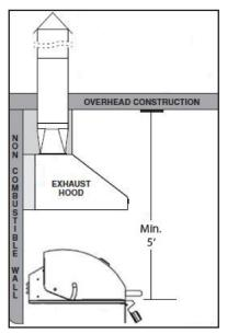
**Combustible Overhead Construction:** Exhaust hood required.
