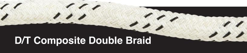
D/T Composite is a double braided rope with the inner core made of Plasma® and the outer sleeve of polyester. D/T Composite has very low elongation, high strength and the feel and handling of polyester double braid. It is identified with three external black markers.
