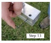
Tighten the set screw and repeat for the other top perch rod.
