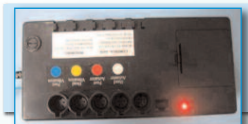
Figure 4: A flashing red LED indicates the control box has received the remote control signal
