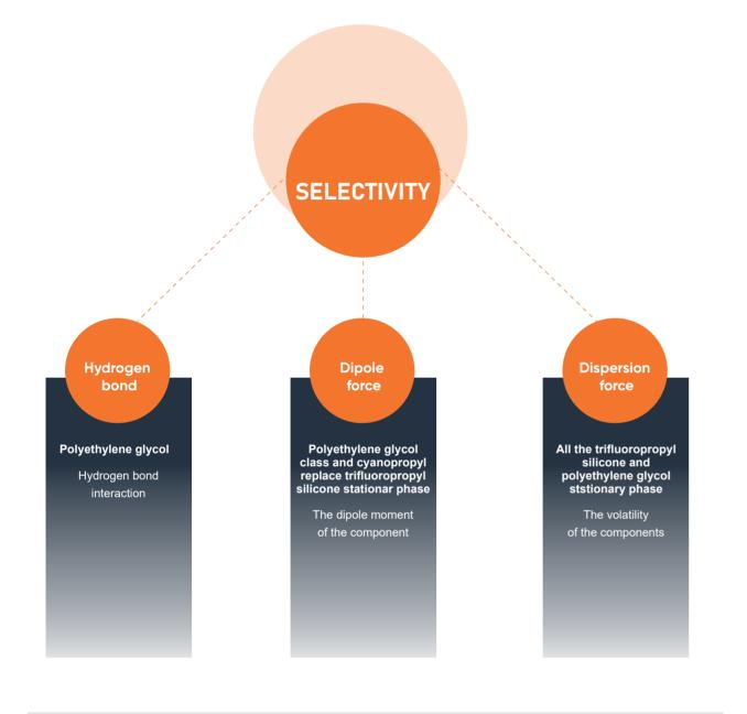
> The selectivity and polarity of stationary phase should be considered, because selectivity is the ability of a stationary phase to distinguish between two component properties (chemical or physical), while polarity depends on the structure of the stationary phase. The selectivity is shown in the following Figure and Table 5.1, and the polarity is shown in Table 5.2.
