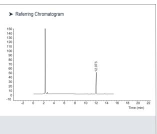
· Possible sources of ghost peaks: sample, solvent, injection needle, gas cylinder, gas purification pipe, gas pipeline, inlet, column, detector. • Using another GC FID but the same column to do the same batch of samples has no problem, exclude the problems of solvent,
