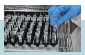
2. During the cleaning process of sample vials, a specially designed basket rack is used, with each sample vial having a dedicated cleaning nozzle. This ensures that the incoming water effectively flushes out any contaminants. The outer surface of the vials is subjected to a circulating rinse using upper and lower spray arms, enabling a 360-degree cleaning of the sample vials. This ensures that even hard-to-clean sample vials are thoroughly cleaned.
