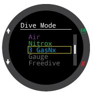
When changing to or from Gauge or Freedive Mode, the decompression tissues are cleared. This is because when in these modes the Tern does not know what gas you are breathing, and therefore cannot track inert gas loading. Plan repetitive dives accordingly.
