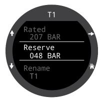
A "Reserve Pressure" warning will be generated when the cylinder pressure falls below this setting. The default setting is 50 bar.
