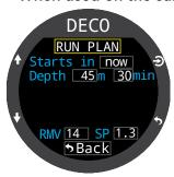
Enter the expected surface interval, bottom depth, bottom time, respiratory minute volume (RMV).
