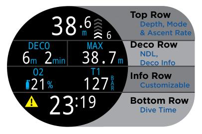
The Standard screen layout has four rows and provides the most information on the screen, though with a smaller font size.
