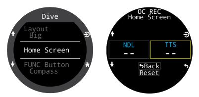
The Big layout allows for customization of the right info row slot only because the left slot is taken by NDL which cannot be permanently obscured.
