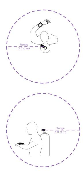
Install transmitter on 1st stage HP port
