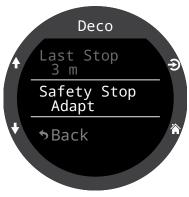
When using the Adapt setting, a 3 minute safety stop will be used, unless the dive exceeds 30m (100ft) or the NDL falls below 5 minutes, in which case a 5 minute safety stop is used.
