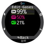
The Edit Gases menu is available both at the surface and while on a dive. Note that changing the gases you have turned on during a dive will impact decompression schedule and TTS.
