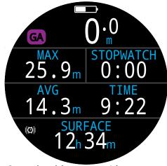
Standard layout - Alternate Gauge Mode configuration.
