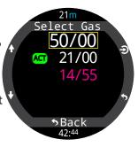
Gases that are programmed but turned off are not used in decompression calculations during a dive or in the dive planner.
