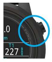
The function (upper right) button is a customizable shortcut that makes accessing your most used functions on the Tern a little easier.
