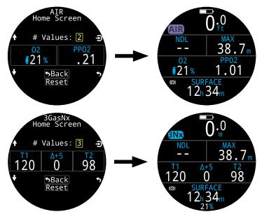
The right slot of the Info Row in the Big layout, and the right Deco Row slot in standard mode are also customizable.
