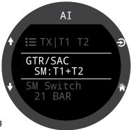
GTR/SAC is only based on one cylinder, or on two cylinders in sidemount configuration. Note that for sidemount the cylinders must be of identical volume for SAC to be accurate.
