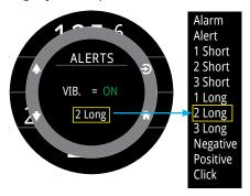
Use the up and down arrows to select an alert and press select to test it.
