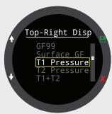
CHANGE GF99 now displays in yellow when above GF High (and still displays in red when greater than 100%).
