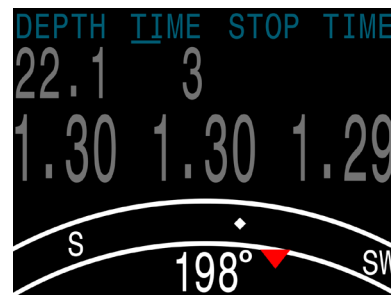
When facing the opposite direction, the reciprocal heading is shown as a red triangle
