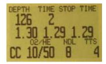
The computer has automatically switched to the high setpoint. This can be disabled if automatic setpoint switching isn't required.
