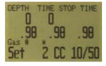
Flipping through the gasses available in the "Select Gas" menu item shows that we have three open circuit gasses available.
