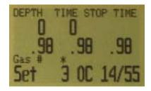
Automatic decisions of when to switch gasses for the TTS calculation means that it is very easy to set up your CC and OC gasses. There is no need to enter a depth or a PPO2 to switch point. There is no need to keep track of which gasses are turned on and of in which mode.
