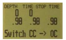
These are the gasses that will be used to estimate TTS in the event that you switch to open circuit during a dive. The computer will assume that you will switch gasses when the PPO2 of the next available gas is less than 1.6.
