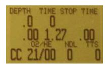
At this point, the system is still averaging the three sensors and is flashing the center sensor. Since it has two sensors that agree the ppo2 is .00, it is voting out the 1.27 sensor. You can see that we have caught the sensor in mid flash.
