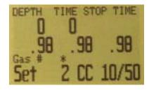
example, when a gas is displayed in the "Select Gas" menu, SELECT will select the displayed gas. When the "Switch Setpoint" menu is displayed, SELECT will switch the setpoint.
