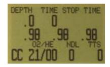
The system will use both of these gasses for our dive when calculating the TTS. It assumes a diluent switch at a PPO2 of 1.0. That means that it will assume that you have switched to an air diluent at 124 feet.
