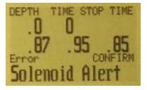
This alarm is a notification that there has either been a very fast ascent for a short period of time, or that there has been an ascent of more than 66 fpm / 20 mpm maintained for over a minute.
