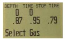
In the "Select Gas" menu, MENU increments the gas number. The right button (SELECT) is used to accept the current choice. In some cases that means save the current value, in others, it means execute the command. For
