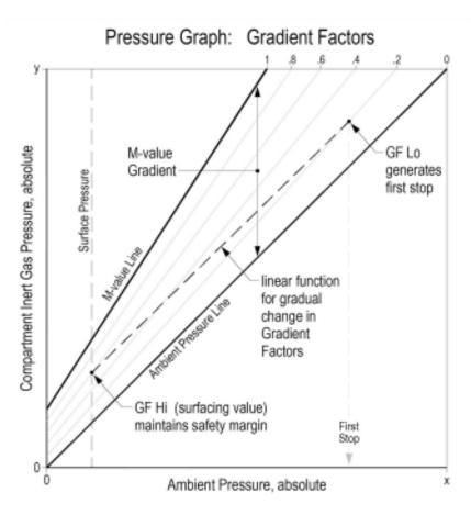
A Gradient Factor is simply a decimal fraction (or percentage) of the M-value Gradient.
