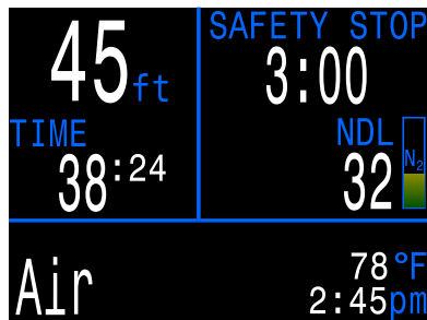
FIGURE 2 The Nitrox Recreational Mode is optimized for Air and Nitrox diving
