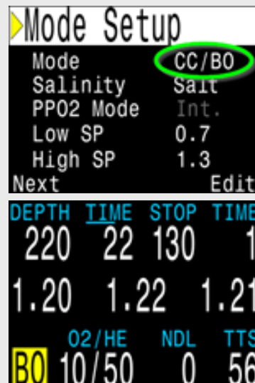
"OC/CC" mode renamed to "CC/BO" for clarity of purpose
