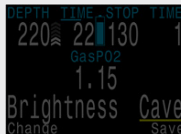
Cave brightness is very dim and thus best suited for dark environments like caves
