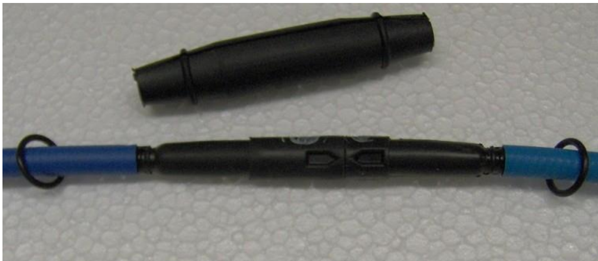
Install O-rings before mating cable.
