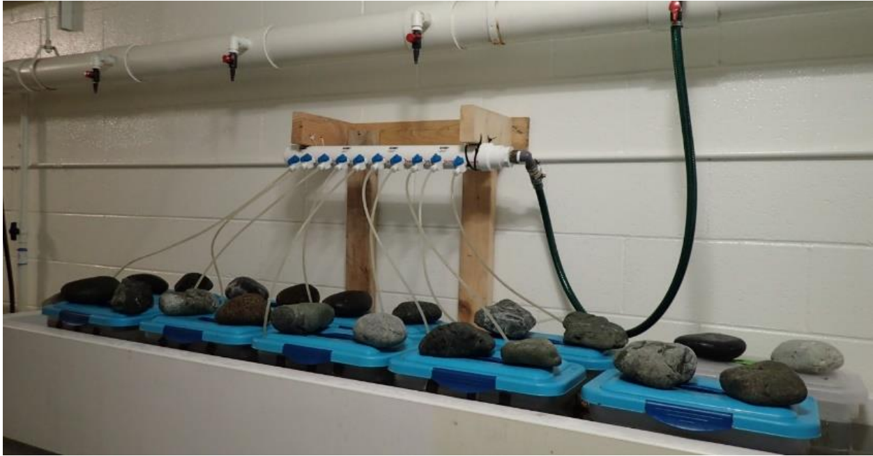
Figure 1. Plastic containers with constant flowing ambient seawater (via a manifold system) which housed individual octopuses; system was designed and fabricated by Chase and Verde (2011).
