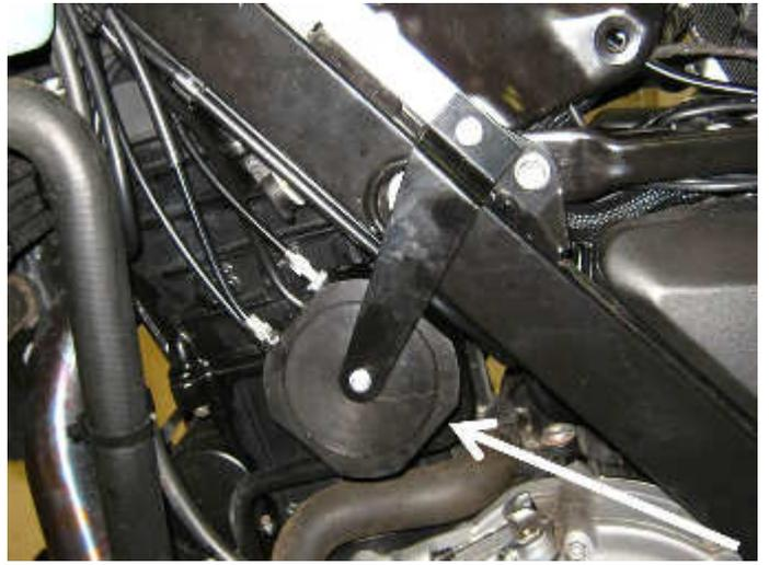
The **Speed sensor (5)** is mounted below the left side of the rear swing arm. The speed sensor detects wheel speed from the slots in the ABS tone wheel (photo below left).
