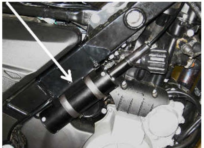
The **CIU or Cable Interface Unit (3)** is mounted on the left side of the bike. It has a new **cable (4)** running from it to the throttle bodies
