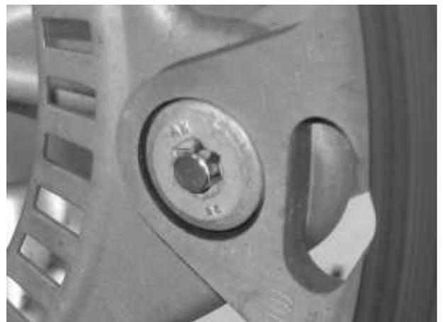
The current F800GS has this new bolt on the front wheel, a T-30 'Torx' fitting and the magnets we use to fit this are 4mm diameter x 5mm long. This design has gone back to the BMW's earlier practice of having a disc carrier bolted to the wheel and then the disc 'floats' on the carrier. We don't know if earlier F800GS models use this bolt on the rear disc as well or use the same bolt used on the current model bikes.
