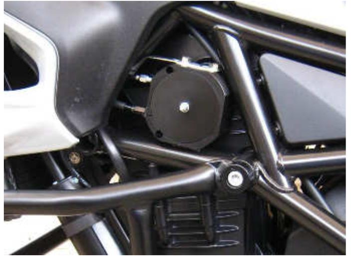
The **Speed sensor (5)** is mounted on left side of the rear wheel, on the ABS wheel speed sensor. Nickel-plated magnets are placed in the heads of the bolts that mount the brake disc.
