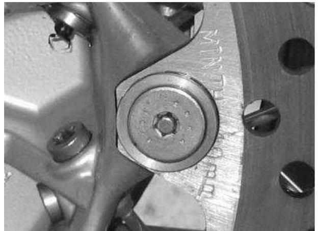
This kit for this model F650/700/800GS comes with magnets to fit the first bolts (flat head T-40). If your bike has different size bolts, please let us know so we can supply appropriate magnets.
