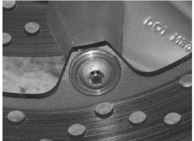
Some current (2008) bikes have flat head bolts. The recess in the head of this bolt is a T-30 'Torx' fitting and the magnets we have to fit this are 4mm diameter x 5mm long. We have seen this bolt on the new (late 2008) R1200GS.
