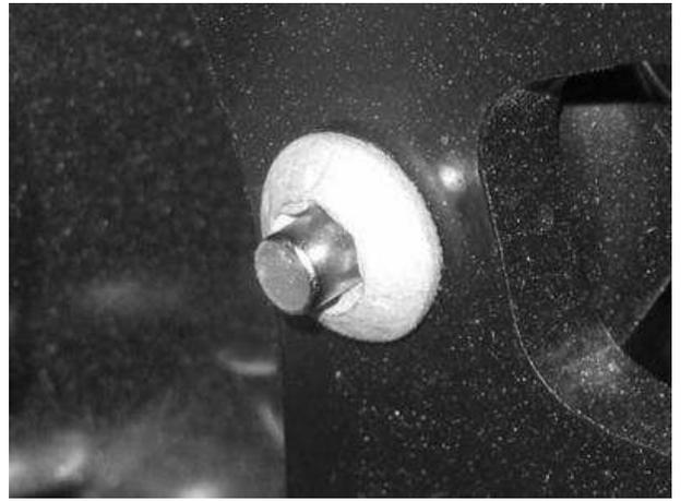
All models that we are aware of from mid '90's to 2007 use this 'button' (rounded) head bolt. The recess in the head of this bolt is a T-40 'Torx' fitting and the magnets we have to fit this are 4.75mm diameter x 4.75mm long. We have seen this bolt in various models, R1100RT, R1150RT, R1150GS, R1100S, K1100RS, K1100LT, R1200GS, R1200S, K1200S, F800ST.
