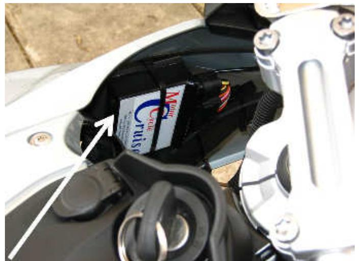
A closer view of the **Electric Throttle Servo (2)**.
