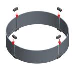
Secure bottom clips to glass panels as shown above.
