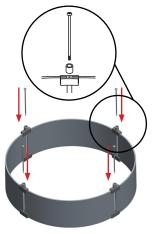
Insert rod through pad, then bottom clip and finally screw into top clip as shown above.
