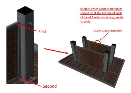
Attach **Panel B** using **Bolt A (4X)** as shown below. 5.
