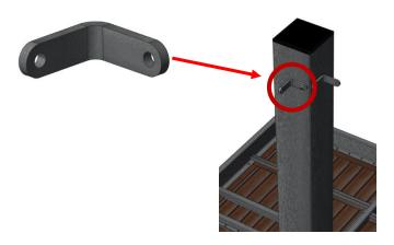
4. Attach <u>Panel A</u> using <u>Bolt A (4X)</u> to legs as shown below. Attach bottom of panel first with the help of the side support brackets. Next attach top of panel to upper support brackets. Repeat process for opposite side.
