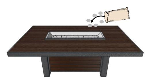
DO NOT OPERATE CRYSTAL FIRE PLUS BURNER WITH GLASS COVER IN PLACE
