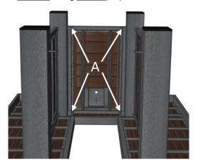
6. Attach Center Support, as shown below, to the bottom of the fire pit using Bolt A (4X). NOTE: Drainage holes on *Center* Support piece must be facing down towards the surface on which you will be placing your fire pit.
