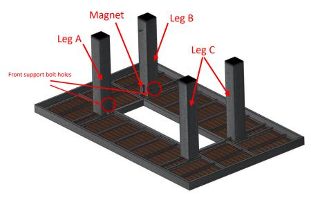
Attach <u>Corner Support Brackets</u> to all corners of legs as shown below. Attach <u>4X</u> brackets to each <u>Leg C</u>, attach <u>3X</u> bracket to <u>Legs A and B</u>. Brackets attach using <u>Bolt A (1X)</u>. Tighten bolts to help stabilize side panel when attaching.
