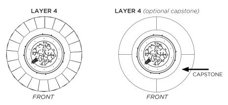
**OPTIONAL CAPSTONE SETUP:** The BRON52-K has an optional captone. The capstone can be place on top of layer 3 (replacing the brick of layer 4) or on top of layer 4. When using the optional capstone ensure that the burner plate is one layer below the capstone.
