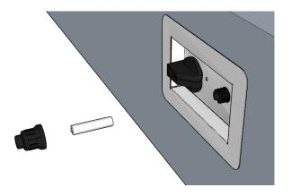
6. Remove tie(s) for gas line and set into place.
