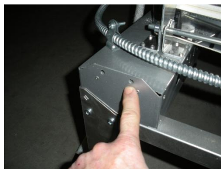
Locate the 2 holes in the right rear floor base. Of these 2 holes, you will be placing the other end of the spring into the inner most as indicated.
