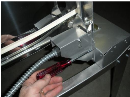
Attach the power interrupt switch bracket to the inside, back left floor base with the included screws as shown.
