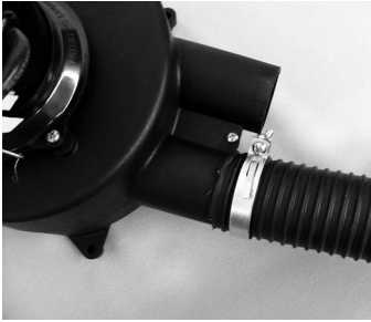
High temperature black flex hose attachment to blower housing
