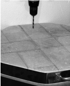
Drill holes in kiln lid with drill bit provided
