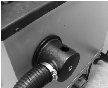
Side kiln mount of collector cup
