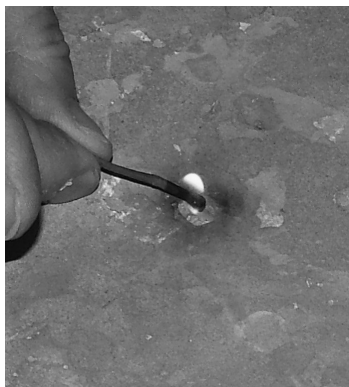
Flame is pulled into the kiln
