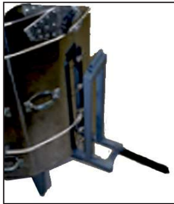
Position kiln floor and rings on stand with hose clamps on the stainless steel jacket facing the back supports. If your kiln is stackable, plug in twist 'n lock interbox plus and receptacles.
