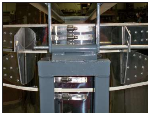
Position armlifter holes to match back of vertical back support holes and holes of lid. Insert stiffening strut through holes and lock in place with cotter pin.
