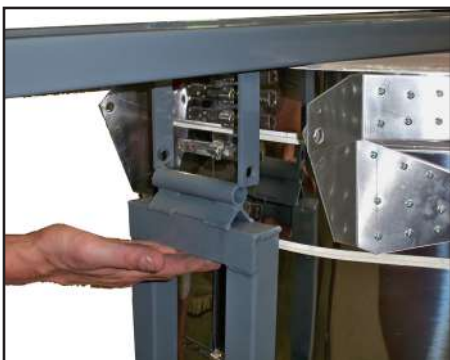
Position armlifter holes to match back of vertical back support holes and holes of lid. Insert stiffening strut through holes and lock in place with cotter pin.
