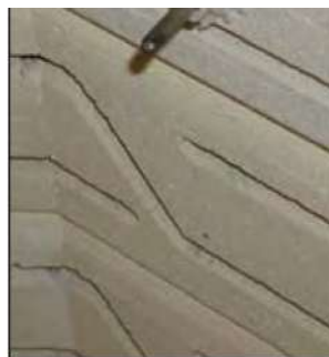
Thermocouple will show through brick wall at a maximum of 1". Pack kiln sitter hole with ceramic fiber to seal it.
