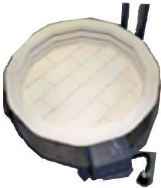
Position kiln floor and rings on stand with hose clamps on the stainless steel jacket facing the back supports. If your kiln is stackable, plug in twist 'n lock interbox plus and receptacles.
