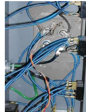
Connect wires to back of Electro Sitter just like the connections to the back of the kiln sitter.
