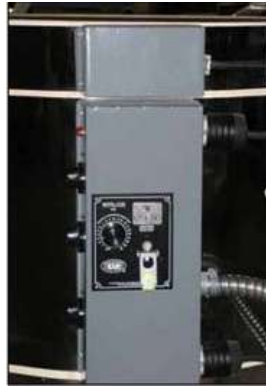
Detach screws from kiln sitter plate
