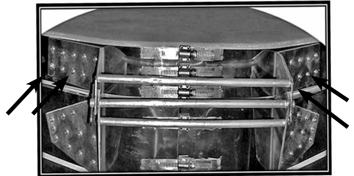
Repositioning Lid when Thermal Expansion Occurs
