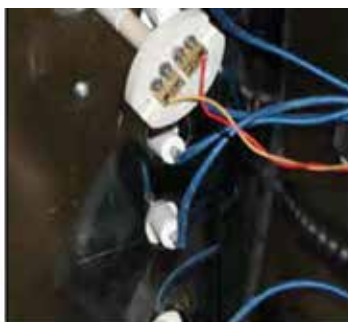
Insert thermocouple through kiln sitter hole
