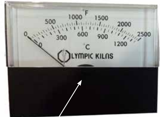
Adjust setscrew for calibration
