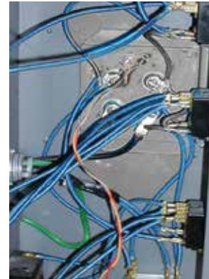
Connect wires to back of Electro Sitter just like the connections to the back of the kiln sitter.
