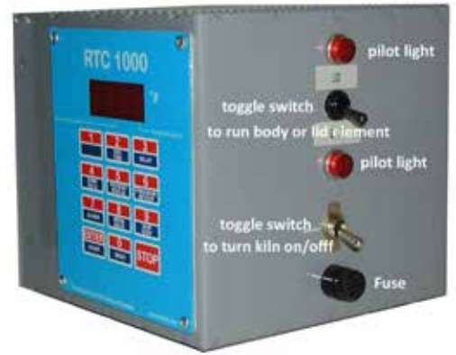
120 volt glass kilns – top toggle switch for element operation – must be in the Up or Down position for element to heat
