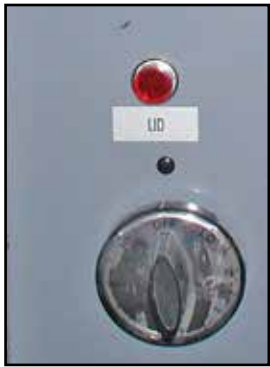
240-208 volt glass kilns – infinite switch for lid element operation
