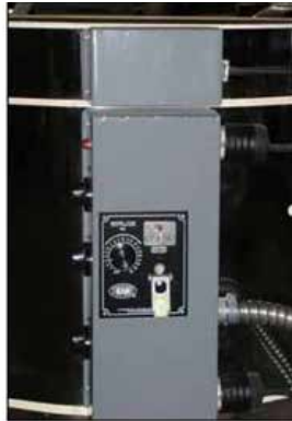
Detach screws from kiln sitter plate
