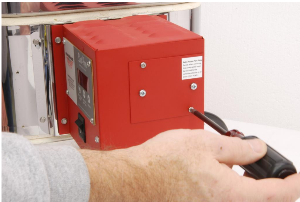
Place the relay access plate back into the access port as shown and secure with the included screws as shown. Relay replacement is now complete. That was easy!
