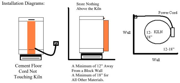
Kilns must have an Air Space Under the Kiln. Kilns Cannot sit directly on a floor or any surface. Use a kiln stand or concrete blocks with the holes up and down at a minimum. Small Table Top Kilns can be used with a kiln stand or the kiln bricks supplied as long at the material under the kiln is not combustible.
