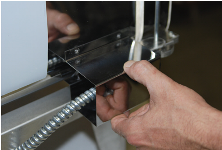
Place the Power Interrupt Cover Plate Against the Oven Body as Shown
