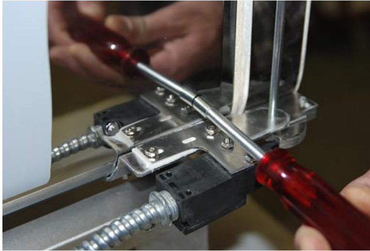
Remove the two #6 Power Interrupt Cover Plate Mounting Screws from the Oven Body
