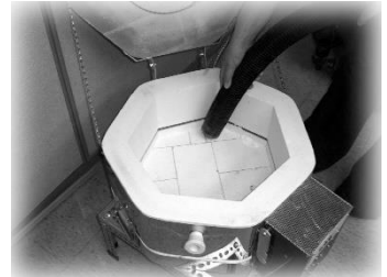
Vacuum any loose debris
