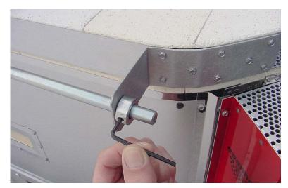
Center the Dyna-Lift link on the lid handle rod. Once centered move the collar clamps up to each side of the link and tighten with the 1/8" allen wrench.
